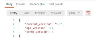
In the bottom half of the window is the response from the server which in this case is various versions. This specific endpoint does not required authentication and can be accessed by anyone. This is not the case for most endpoints where token authorization is handled by rails. One can retrieve a token with Postman by logging in through the login endpoint but there is an easier way to test endpoints if you are running a local server.
